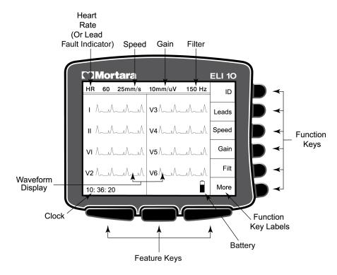
**NOTE**: Device display defaults to real-time ECG view.
